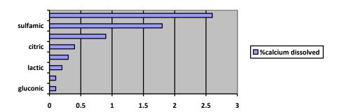
The graph shows competitive descaling profiles of various chemistries. GreenCat outperforms other products while being a non-regulated DOT class, phosphate free and VOC free.
